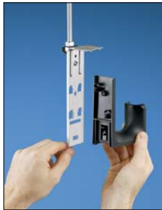
Align snap lock attachment of J Hook with holes in chosen bracket and snap J Hook into place
